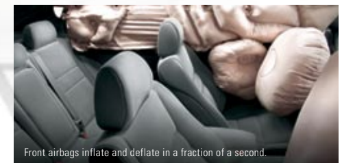
Front airbags inflate and deflate in a fraction of a second.
