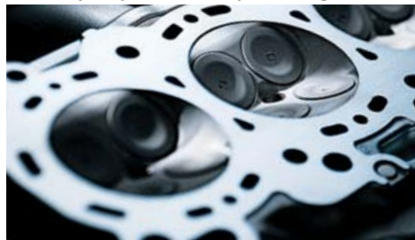
4 valves per cylinder for easy breathing.
